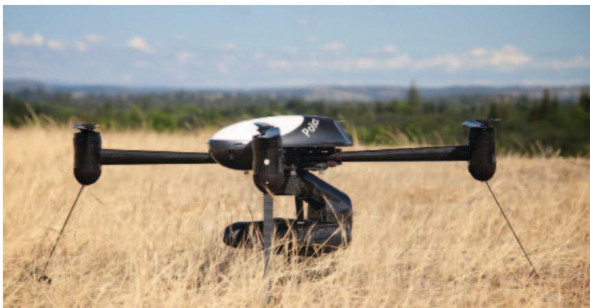
The Draganflyer X4-ES model is a five-pound, four-rotor helicopter. With the capability of adjusting itself, the X4-ES "tilts" forward during windy conditions or when flying to another location, the same as a real helicopter, but the camera remains in position automatically.
